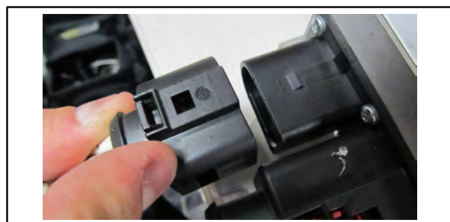
Figure 9-3 Remove the Small Connector
