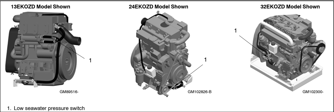
Figure 1-10 Low Seawater Pressure Switch Location
