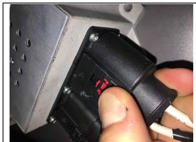
Figure 9-5 Remove the Large Connector
