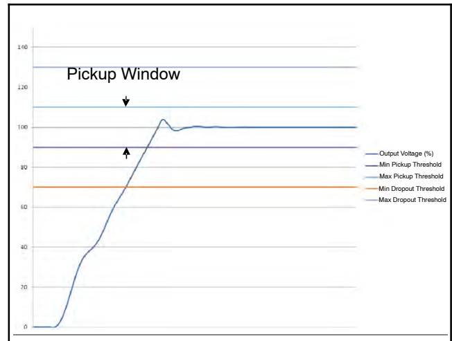
Figure 12-2 Pickup Acceptable Voltage Window
