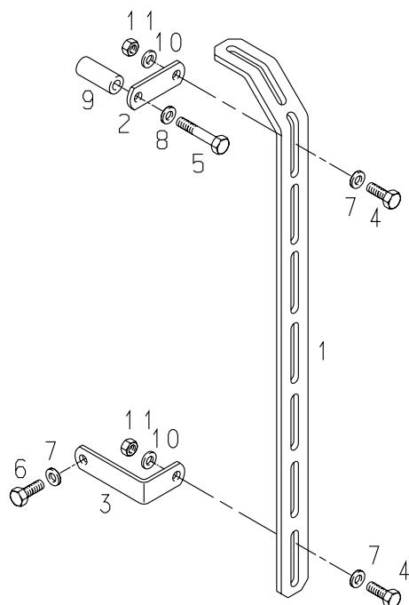
**D 2842 LE410****25-3047****BRACKET FOR WIRING HARNESS****HALTER FÜR KABELBAUM****SUPPORTO PER FASCIO CAVI**
