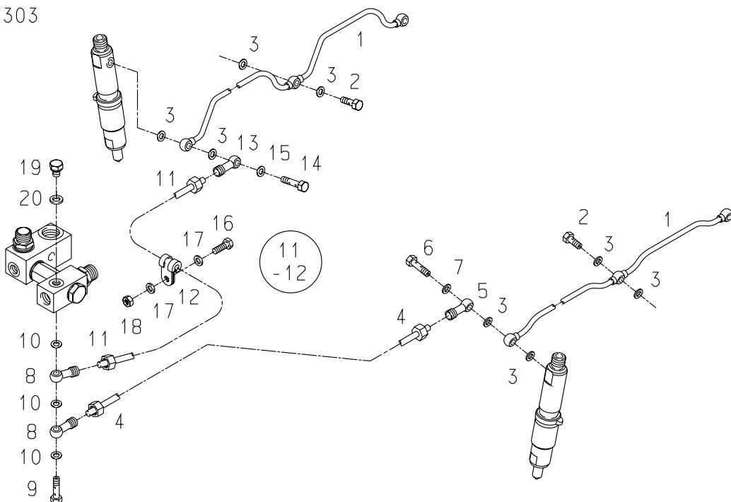
**D 2842 LE410****12-4079****LEAK FUEL PIPE (FOR
