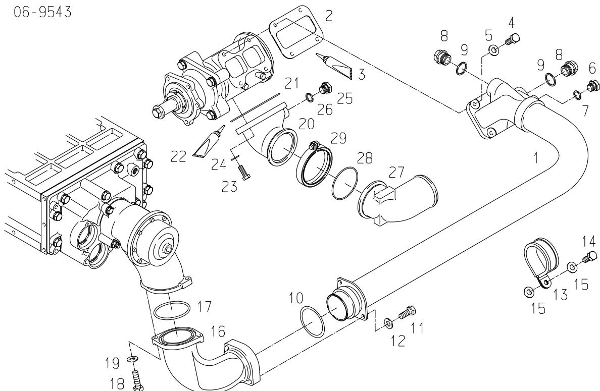
**D 2842 LE410****06-2090****COOLING WATER PIPES
