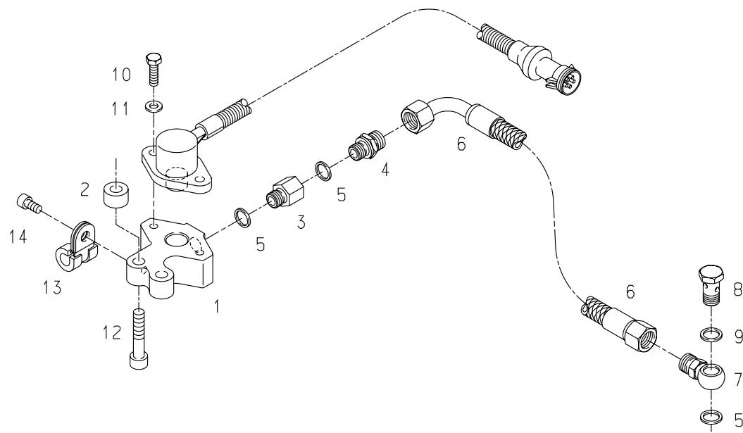
**D 2842 LE410****27-1076****PRESSURE SENSOR****DRUCKSENSOR****SENSORE A PRESSIONE**
