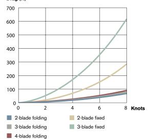
Water drag were measured in a test carried out by SSPA Maritime Consulting. Propellers mounted on S-drives were measured. The lower drag produced by the Volvo Penta folding propellers can boost sailing speed by up to 1.5 knots.
