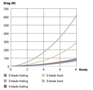
Water drag were measured in a test carried out by SSPA Maritime Consulting. Propellers mounted on S-drives were measured. The lower drag produced by the Volvo Penta folding propellers can boost sailing speed by up to 1.5 knots.
