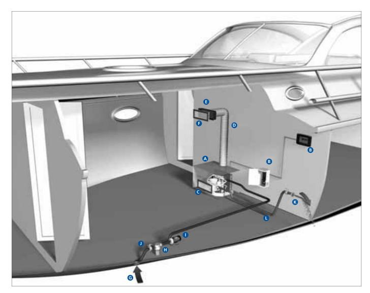
Installation of a BlueCool self-contained unit is quite simple: Each cabin has its own self-contained unit  ${\color{blue} \bf A}$ providing cool air to this cabin. It is controlled by an Air Control unit B which is also located in this cabin. The generated heat is transferred into the sea via the sea water circuit **G** to **L**.
