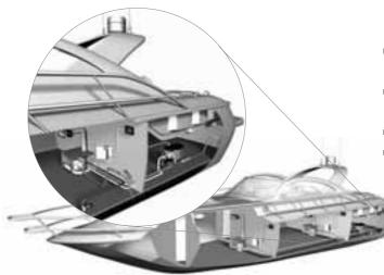
The benefits of a self-contained A/C unit complemented by a compact, high efficient diesel heater.
