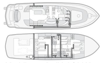
The heater in this 50' motor yacht provides heating for both decks. A combination of convectors and fan blowers is used. For heating sanitary water as well, a Webasto water station could be used to easily integrate a calorifier.
