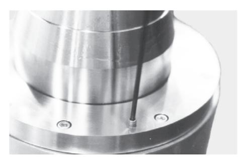
Figure 62. Installing pusher screws
