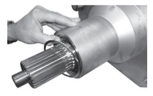
Figure 73. Installing Spiral Lock Retaining Ring
