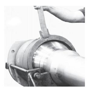
Figure 70. Tightening the Aft Retainer using Special Wrench
