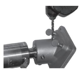
Figure 81. Drill 1/8" into the retainer threads.
