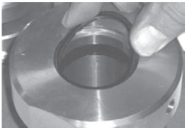
Figure 89. Install the polypak seal into the guide followed by the wiper.
