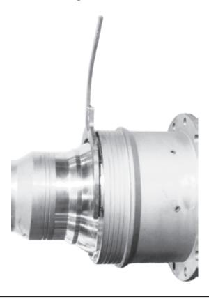
Figure 29. Unscrewing threaded Aft Retainer
