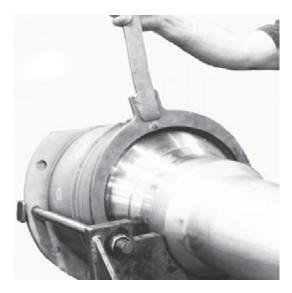
Figure 35. Removing the Aft Retainer using Special Wrench
