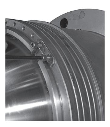
Figure 34. Aft Retainer Ring Lock Clip in the Notch Locking Tab
