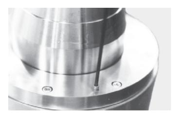
Figure 63. Installing pusher screws
