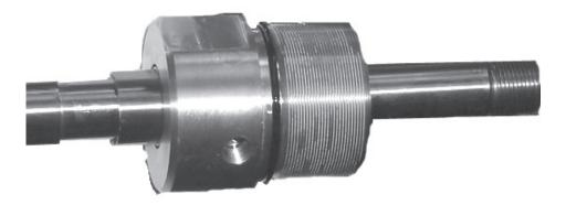
Figure 83. Slide the guide on to the rod.
