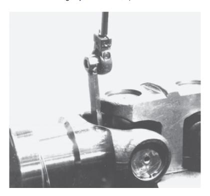
Figure 46. Removing Flex Lock Nut From Input Shaft Using Special Tool T-21093
