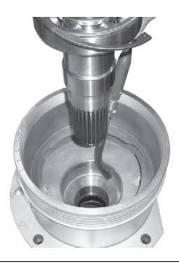
Figure 67. Installing Input Shaft and U-Joint into Socket
