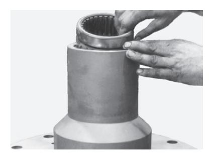
Figure 65. Installing Frozen Forward Socket Bearing into Socket
