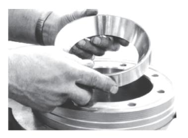
Figure 55. Installing First Bearing Cup
