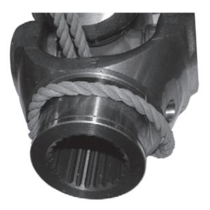
Figure 69. Support U-Joint During Installation of Thrust Tube into Thrust Socket
