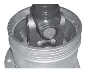
Figure 43. Removing Shims, O-ring, Packing, and Forward Retainer
