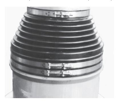
Figure 75. Boot Secured With Three Circle Clamps
