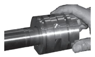
Figure 92. Thread the piston back on to the rod.
