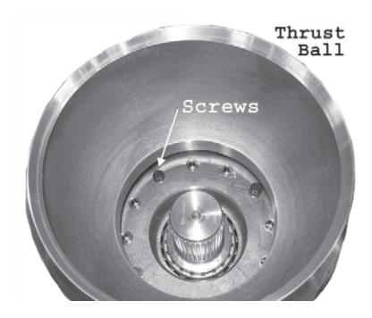
Figure 36. Rotate Thrust Tube Assembly so Ball is Up, Remove 12-point Capscrews
