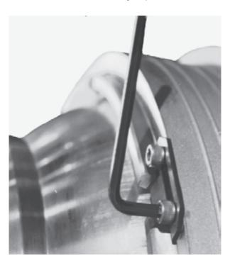
Figure 28. Removing the Safety Clip Around the Aft Retainer
