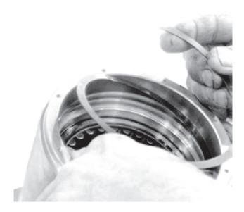
Figure 54. Installing Rear Bearing Spiral-Lock Retainer Ring
