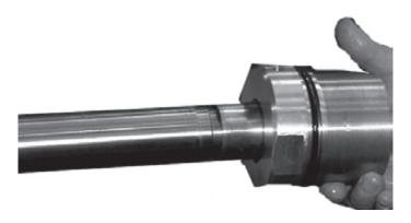
Figure 90. Slide the guide on to the rod.
