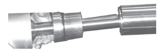
Figure 95. Insert the piston rod assembly into the tube.
