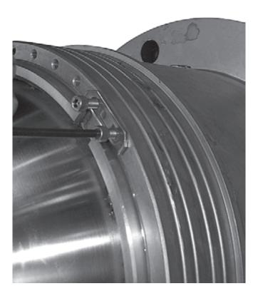
Figure 74. Aft Retainer Ring Lock Clip in the Notch Locking Tab
