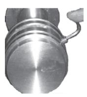
Figure 94. Tighten the setscrew.
