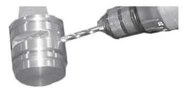
Figure 93. Drill 1/8" into the retainer threads.
