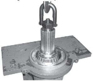
Figure 56. Installing Propeller Shaft Assembly into Thrust Tube
