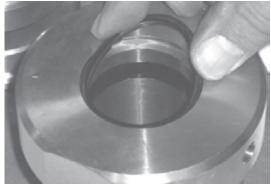
Figure 82. Install the polypak seal into the guide followed by the wiper.
